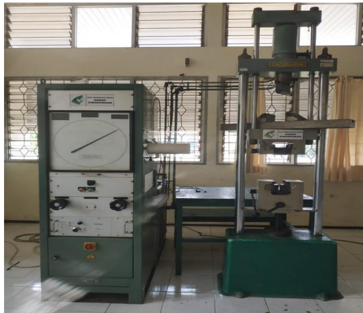
Figure 5. Universal Tensile Testing Machine with The Brand Hidraulic Universal Material Testing Machine Made in China (Source: Civil Engineering Concrete Labor Padang State University)
